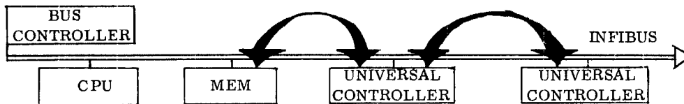
Figure 9-1. CPU-Independent I/O Transfers
